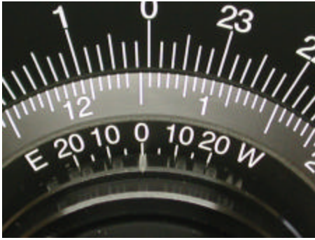
Time Meridian Indicator mark zeroed to Meridian Offset Scale.
